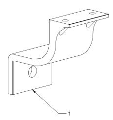
3) Refer to these instructions to install Inline Design square or round tubing and additional hardware Note: If using a round handrail, position the round saddle adapter on top of the flat saddle before attaching handrails.
